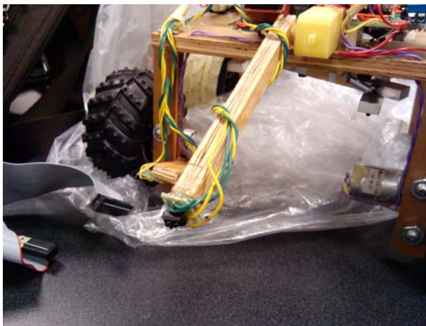
Fig. A-9 Hole sensor a) mechanism b) hole sensor motor attached to base
