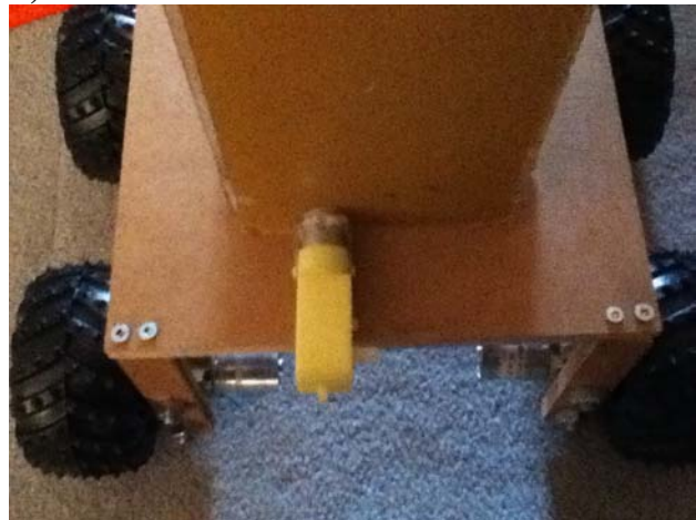
Fig. A-9 Hole sensor a) mechanism b) hole sensor motor attached to base
